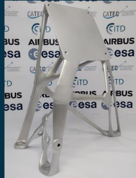
Additive manufacturing for novel structural components (CATEC) (demonstrated in JUICE)
