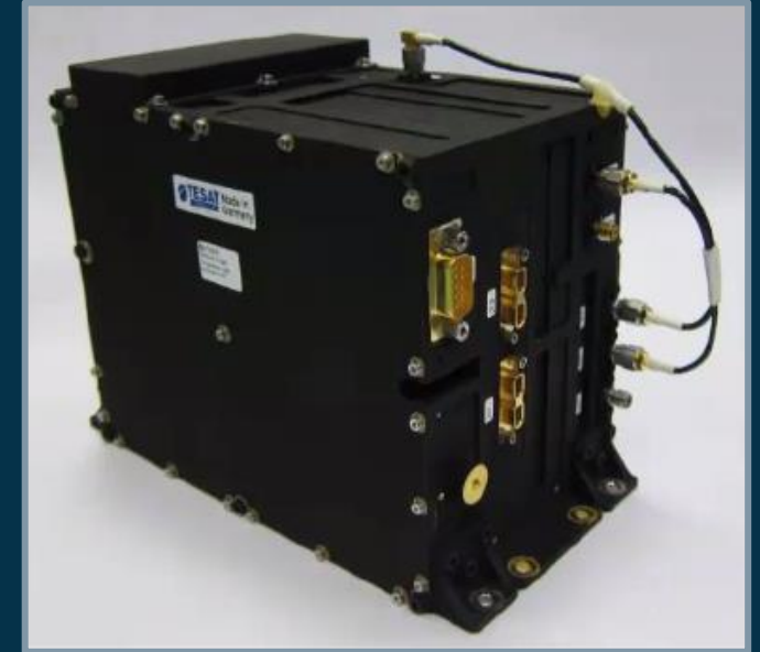
Reconfigurable telemetry transmitter for Earth observation satellites (TESAT)
