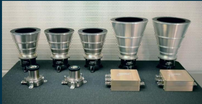
Miniature Active Pixel Sensor based Star Tracker Engineering Qualification Model (TERMA)
